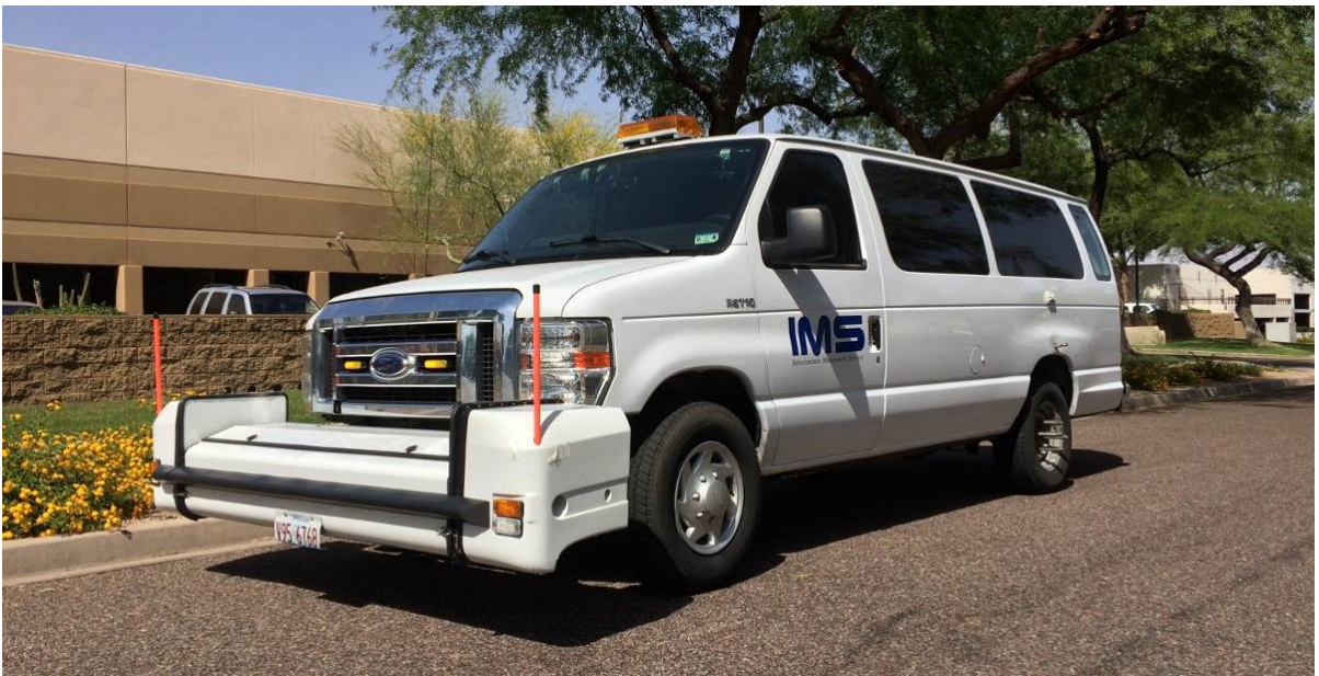
Figure 5 – Laser Road Surface Tester (Laser RST)
